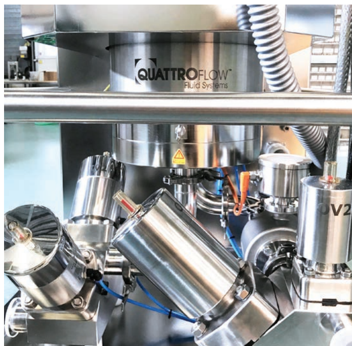
An HP-RFC column that is properly packed with resins enables better separation and resolution of the target proteins. Playing a critical role in the resin-packing process, due to their sensitive handling of the delicate or rigid resins, are Quattroflow™ Quaternary Diaphragm Pumps.
